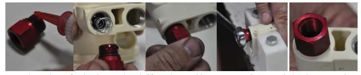
Place 2 drops of Red Locktite on thread of fitting (1541B --blue or 1541R--red) .Screw in by hand to start. Tighten using ¾" closed end wrench until O-ring is fully seated and fitting is tight. Tighten and allow Locktite to dry. NOTE: Locktite and time to dry are essential. Accidental removal and improper installation of the fitting can cause the air control lever to malfunction.
