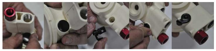
Press in vacuum plug in the hole below air inlet on housing by hand. Slide in speed control and plunger until fully seated.
