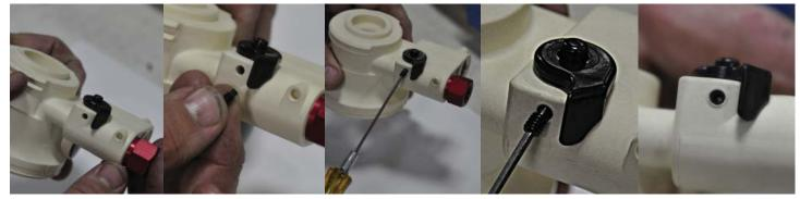
Rotate Speed control to OFF/BACK position. Screw in 8/32 full dog set screw until speed control has slight drag and then back out ¼ turn.
