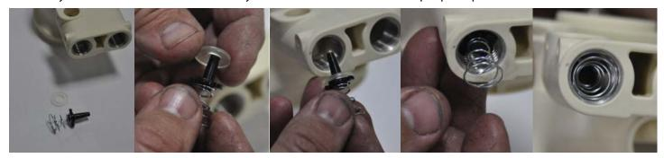
Install Air control (1530 includes valve, washer, spring & air control) in housing. Slide vinyl washer on tip of valve with spring attached. Insert all 3 parts into intake on left side of housing (1515).
